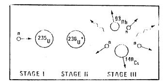
FIG. 1.1: Graphical representation of neutron induced fission in Uranium-235. The fission products Rubidium-93 and Cesium-140 are shown here although other fission products may emerge. Three high energy fission neutrons (n) and other radiations are also shown.
